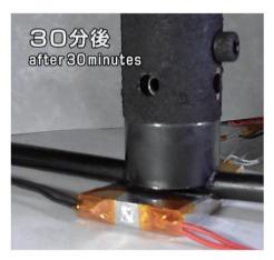
Nail penetration No ignition in either test
