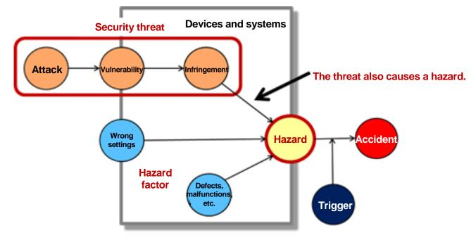
Source: Created on the basis of the SESAMO project SECURITY AND SAFETY MODELLING FOR EMBEDDED SYSTEMS Fig. 10 Model of security problems affecting safety
