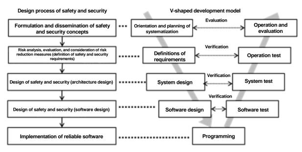
Source: Introduction of Safety and Security Design of Connecting World Fig. 11 Verification and Evaluation of Safety and Security Design
